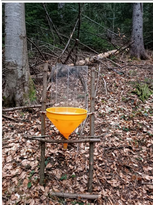
Figs 2, 3. Traps used in the coniferous forests of the Carpathian National Nature Park during the fieldwork in 2023 and 2024: 2 — combined barrier trap; 3 — transparent Polytrap-type barrier trap.
